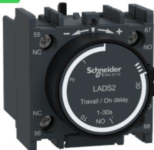
Time delay contact block, TeSys Deca, 1NO+1NC, on-delay 1-30s, front, with  $40 \pm 15$  ms switching time between NC opening and NO closing
