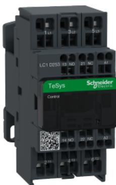
Contactor, TeSys Deca, 3P(3 NO), AC-3/AC-3e, 0 to 440V, 25A, 230VAC 50/60Hz coil, spring
