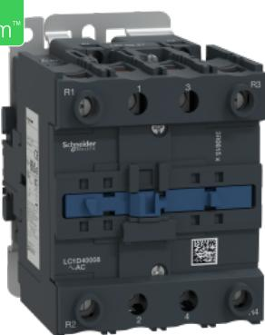
**TeSys Deca contactor, 4P(2NO + 2NC), AC-1 <=440V 60A, 48V AC 50/60Hz coil**
